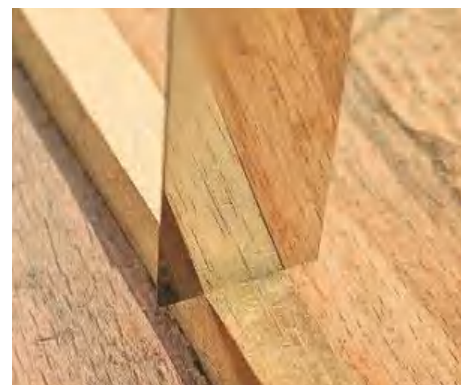
▲ Pic.4 How to get the right angle. The edge is square, but the blade is leaning towards us...
